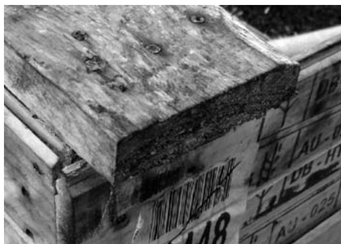
Wooden packaging with heat treatment stamp on crate, but contaminated wood on top
