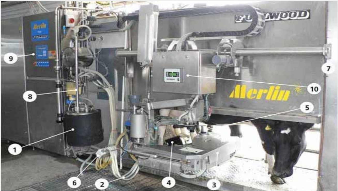
1. Milk receiver can 2. Quarter milk tubes 3. Robotic arm 4. Teat cleaning brushes 5. Scanning laser 6. Milk sensor 7. Feed dispenser (hidden) 8. Milk meter 9. AMS control panel 10. Robotic arm control panel
